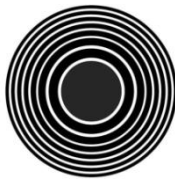
2 MHz array made of eight equiareal coaxial PZT-4 rings
