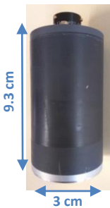
2 MHz array made of eight equiareal coaxial PZT-4 rings
